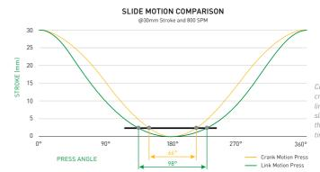
Compared to the crank motion, the link motion keeps the slide on the bottom of the stroke approx. 1.5
