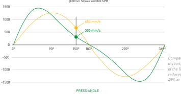
Compared to the crank motion, the slide speed of the link motion is reduced to approx. 45% at 150°
